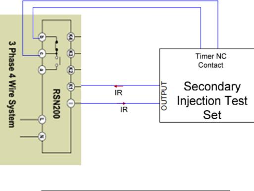
Secondary Injection Test On IDMTL Relay
